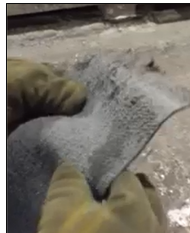
TXP600SILN after being immersed for a few seconds in a molten aluminum tank.
